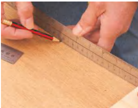
STEP 4. Draw the lower curve on the back by flexing a steel rule or narrow batten between two cramped offcuts
